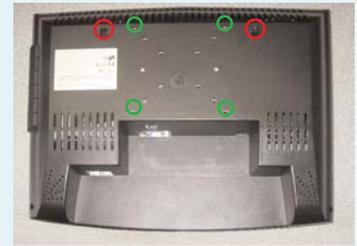
Picture frame style mounting holes (red)
