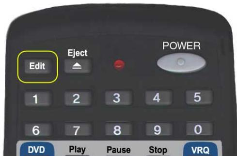
The Edit button is located in the upper left hand corner of your VideoReQuest remote control. The Edit command can be used to edit an unknown DVD or any DVD that looked up incorrectly.
