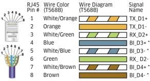
NOTE: The wires marked with a \* are very important for the panel to receive power. A cabled wired using the 10Base-T standard (only 4 pins used) will NOT work.
