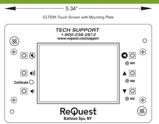
To calibrate the iQ.TS35, remove the front plastic face plate held by magnets. Press the Calibrate button on the left side. Press white squares in sequence. Do not change R49, R48, or R42 from factory settings.
