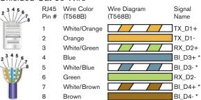
The iQ.TS35 uses a single Shielded Cat 5e cable from the iQ.IMS to supply power, video, and control. This is not an Ethernet network. Do not plug the iQ.TS35 or any of the 8 RJ45 jacks labeled iQ Touch Panels to an Ethernet network or
